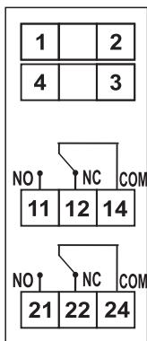
Note- Relay Contacts shown are in power off condition and for relay configuration NC
