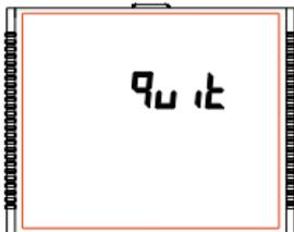
This screen allows user to exit from system "Communication Parameter Selection" setup.
