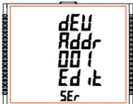
Press "■" to enter into edit mode, prompt for first digit. (Flashing digit indicates cursor position).
