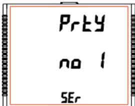
Pressing "▲" key accepts the present value and advances to "Quit Communication Parameters" screen (see section 2.4). Similarly, pressing "▼" key accepts the present value and advances to "RS 485 Baud Rate" screen (see section 2.2).
