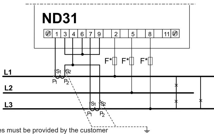
Indirect measurement using 2 current transformers and 2 or 3 voltage transformers in a 3-wire network
