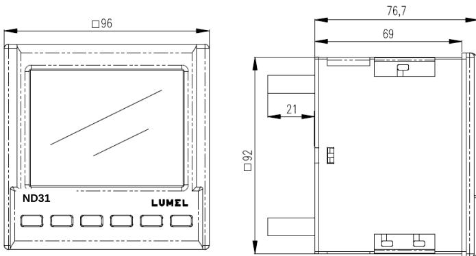
Fig. 3. Overall dimensions of the ND31 meter
