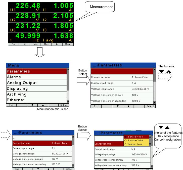
Fig. 19. Screens of Parameters mode
