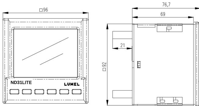
Fig. 3. Overall dimensions of the ND31LITE meter
