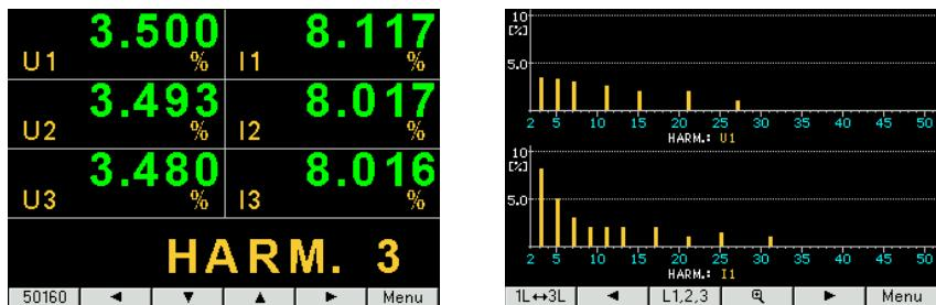
Fig. 16. Screens 11 and 12 - visualization of harmonics
