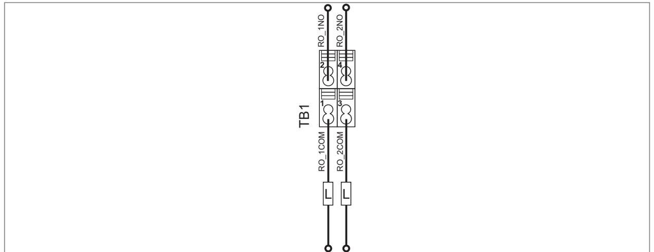
Figure 29 : Relay output wiring diagram (example)
