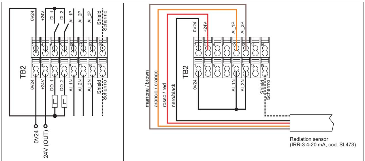
Figure 30 : Regulation circuit Input/Output connection diagram (example)
