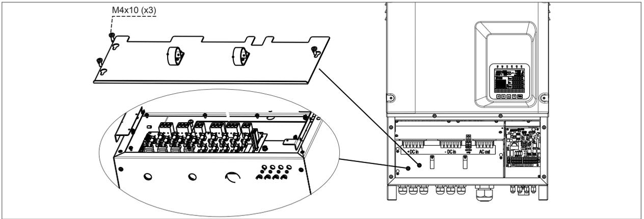
Figure 23 : DC side fuses series PVSA-.k-AE
