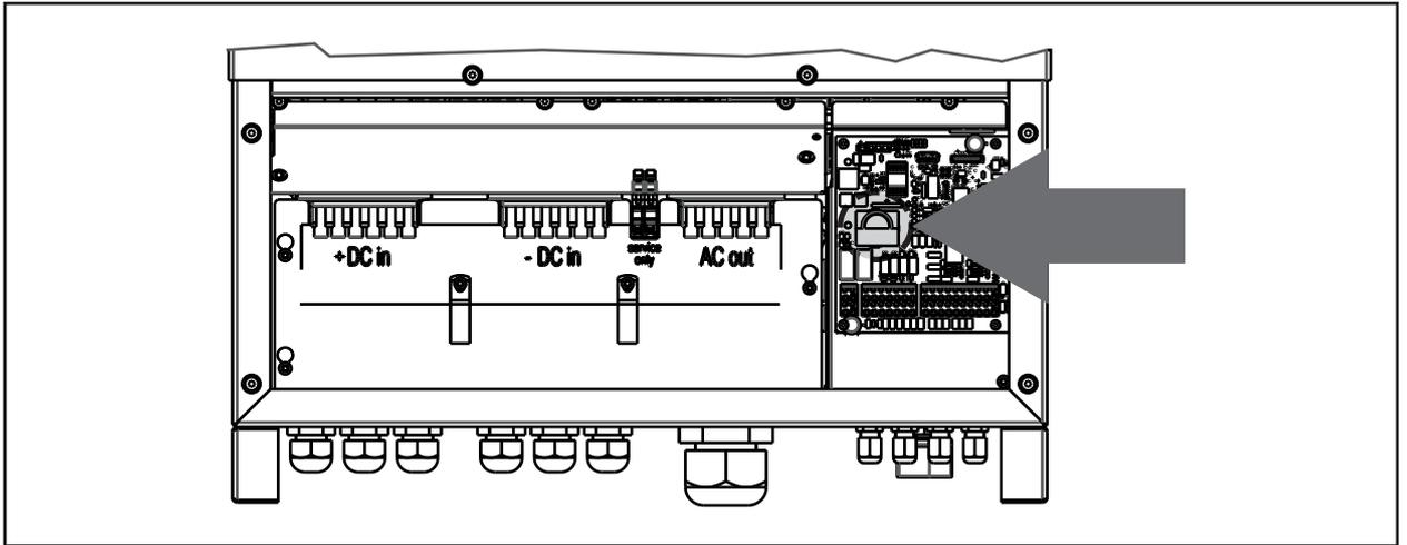
Figure 38 : Position of battery on electronic card
