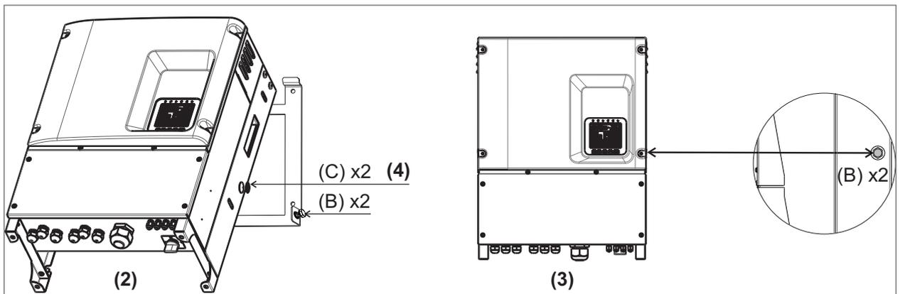
Figure 13 : Fixing the inverter on the bracket
