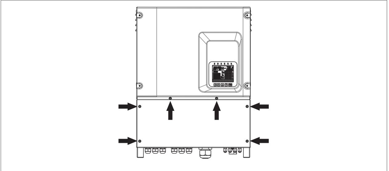
Figure 21 : Fixing of the lower panel
