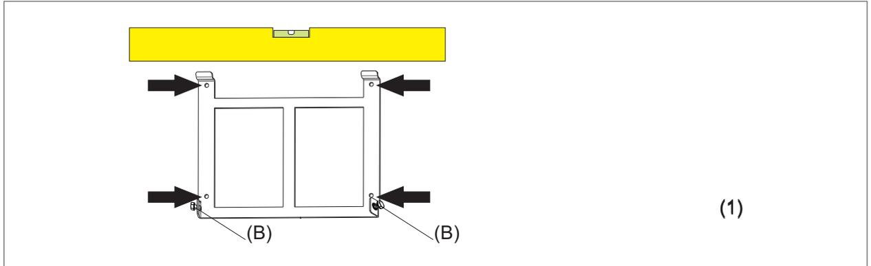
Figure 12 : Mounting bracket fixing
