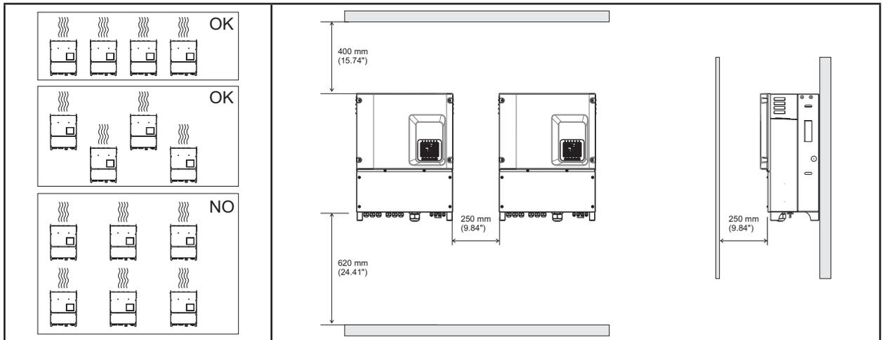
Figure 10 : Free movement of ventilation air and Minimum distances
