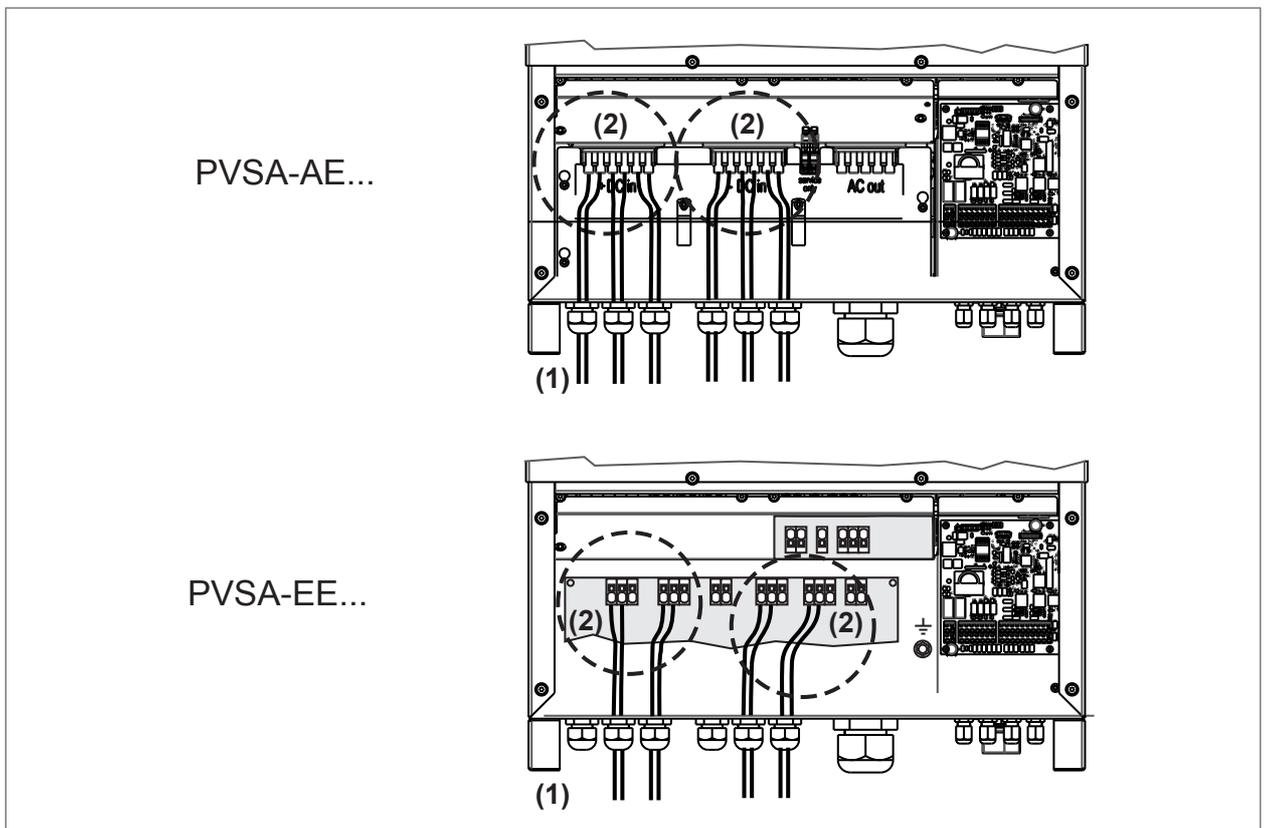
Figure 19 : Connecting to the PV panel
