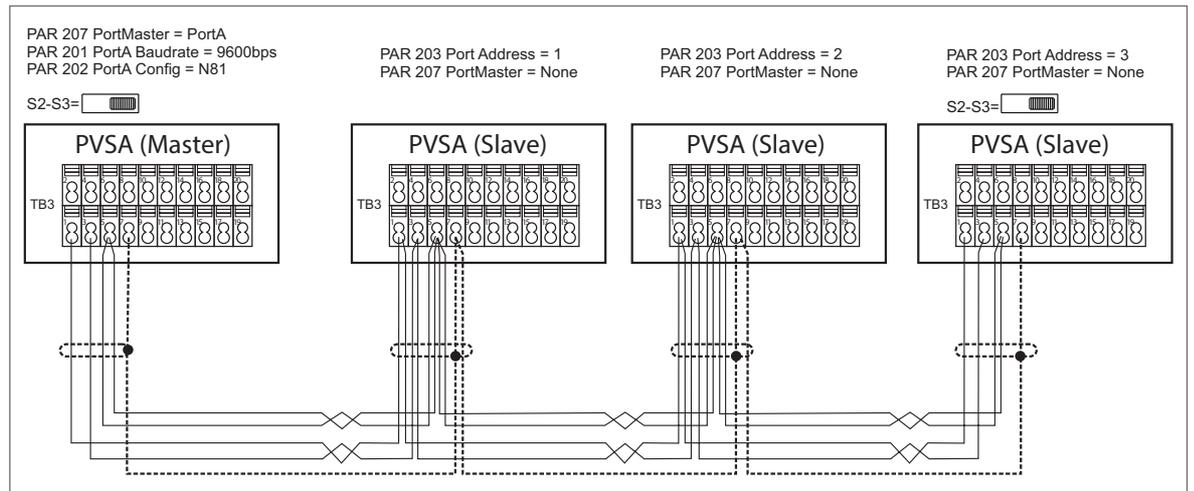
Figure 37 : Example of M/S connection
