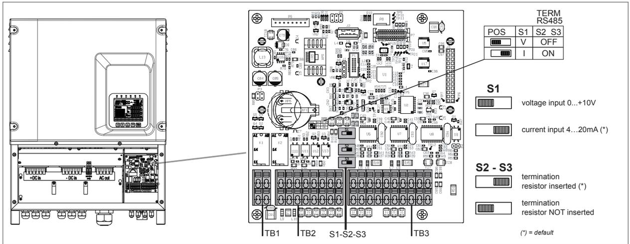
Figure 27 : Regulation and communication terminals. S1-S2-S3 switches
