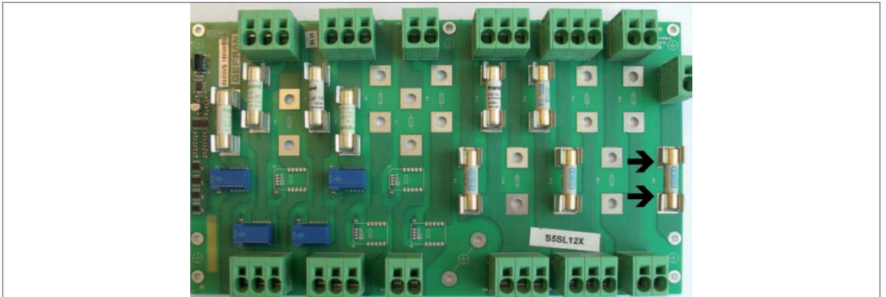
Figure 24 : Ground kit fuse (-F models)
