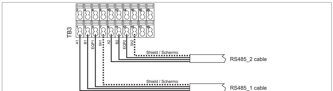
Figure 31 : RS485 connection wiring diagram (example)
