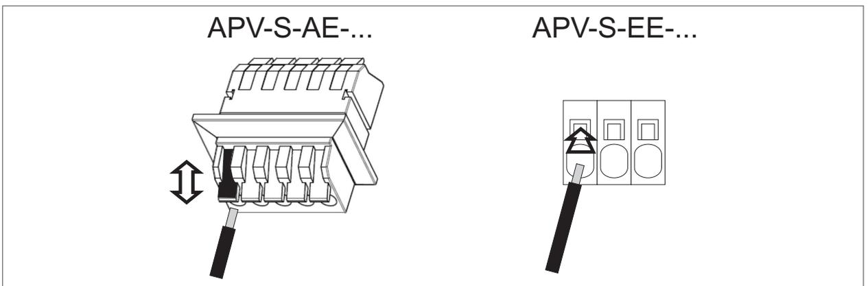
Figure 18 : Insertion of cables in spring connectors
