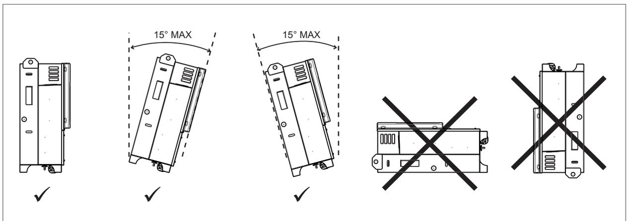
Figure 9 : Installation warning
