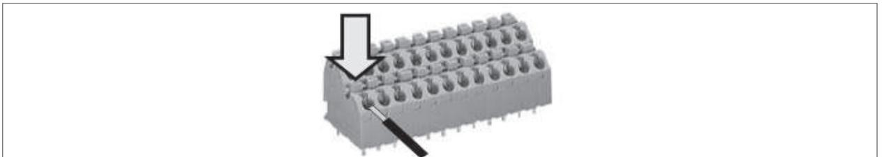
Figure 28 : Insertion of cables in spring connectors
