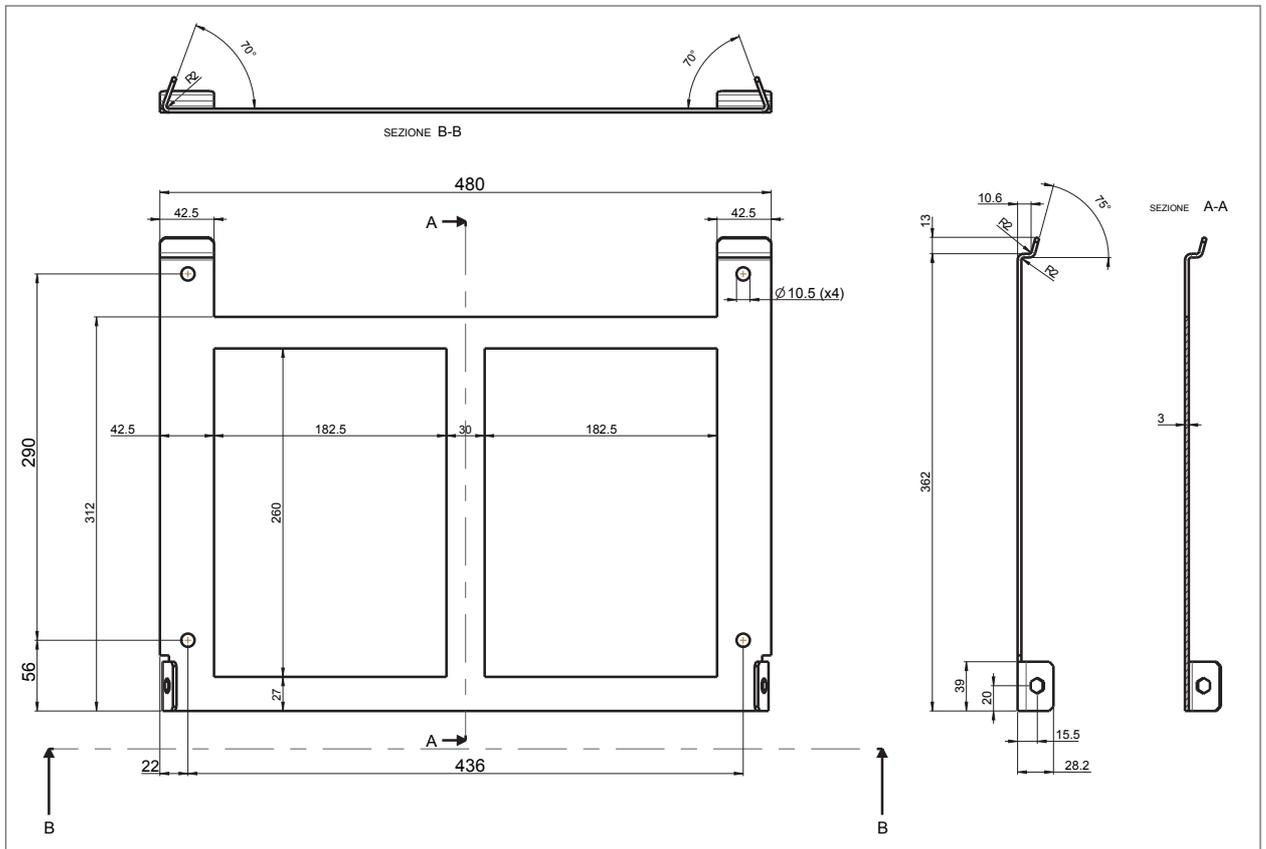
Figure 11 : Wall-mounting bracket dimensions
