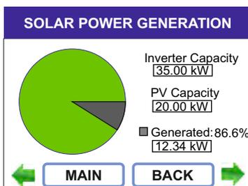
Solar power generation compared to the total PV(Panel) capacity.
