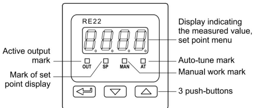
*Fig.6. View of the controller frontal plate.*
