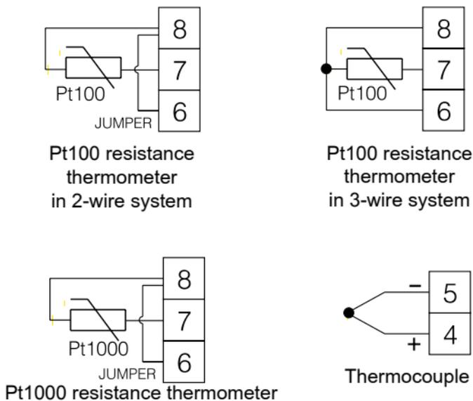
Fig.4. Connection of input signals.
