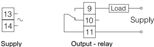
*Fig.5. Connection of the supply and load circuit.*
