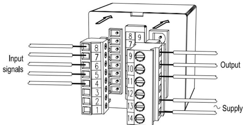
Fig.3. View of controller connection strips.
