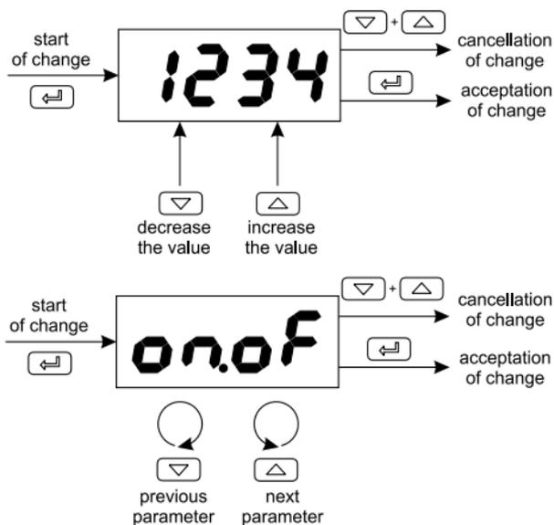
Fig.9. Setting change of numerical and textual parameters.
