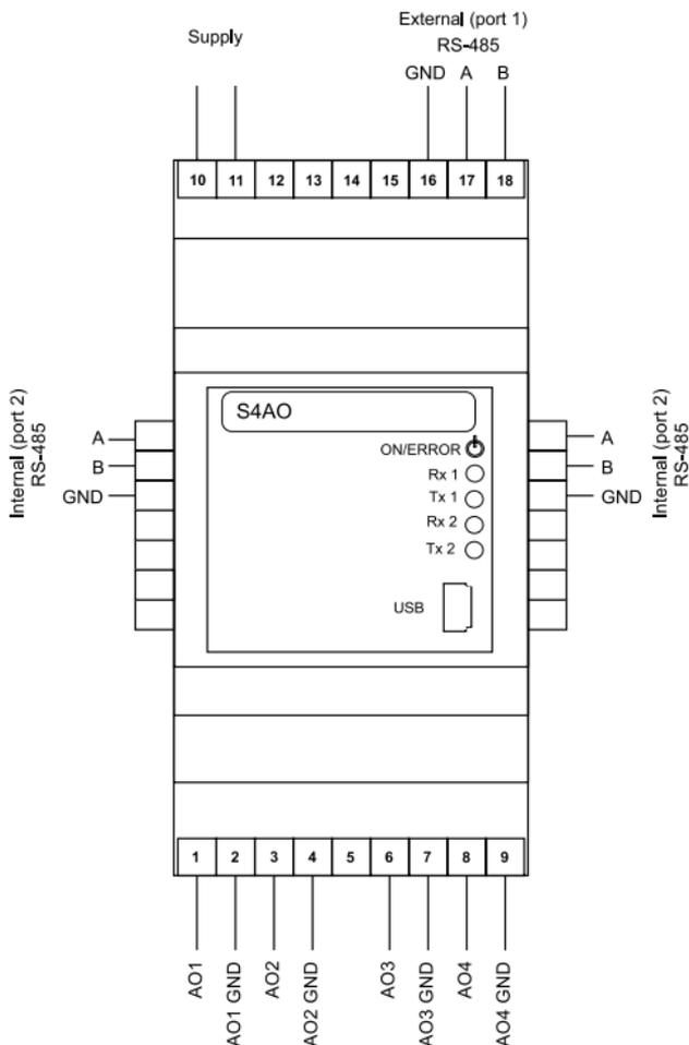
Figure 3: Electrical connections of the S4AO module.
