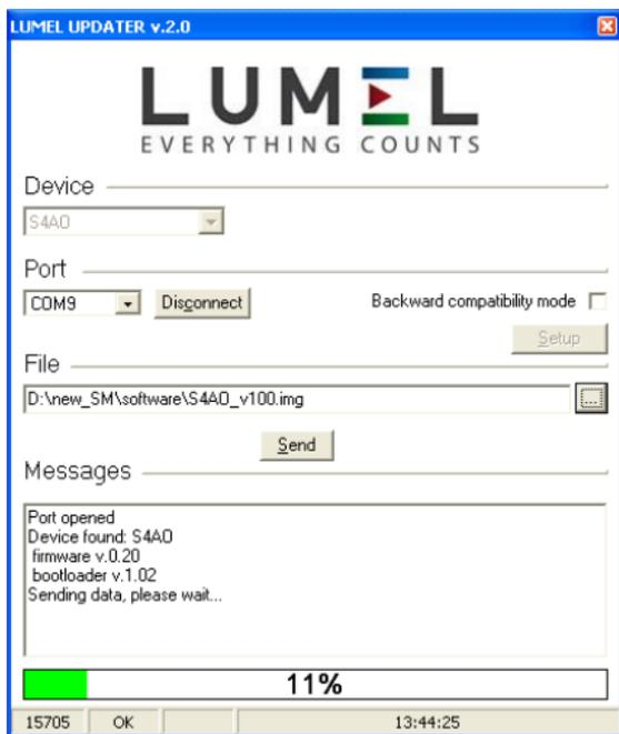
Figure 17: Program window for updating the software
