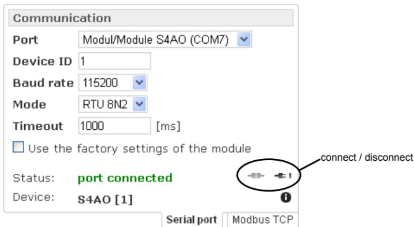
Figure 14: Establishing connection to S4AO module
