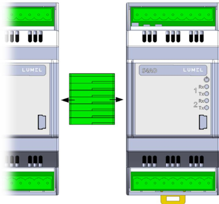
Figure 6: lateral bus connection
