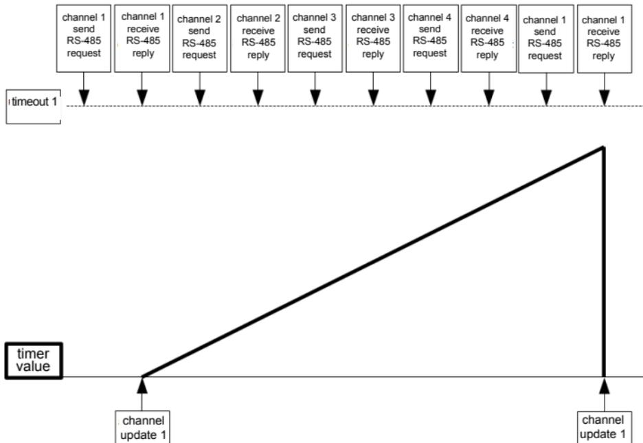
*Figure 11: Master Modbus – Analog output timeout setting*
