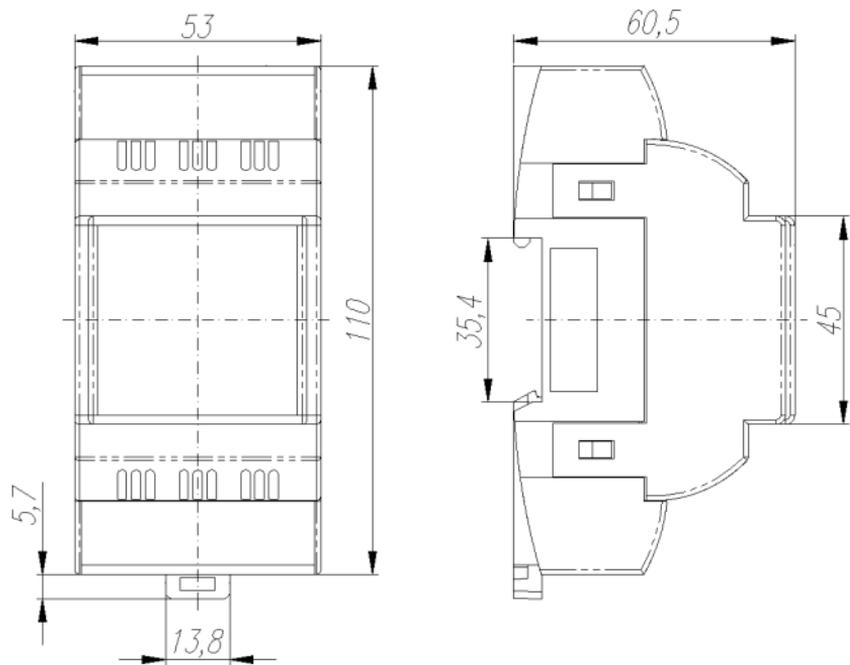
*Figure 2: Module dimensions*
