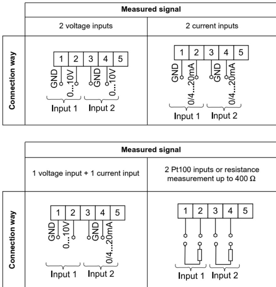
**Fig. 4 Connection way of input signals**
