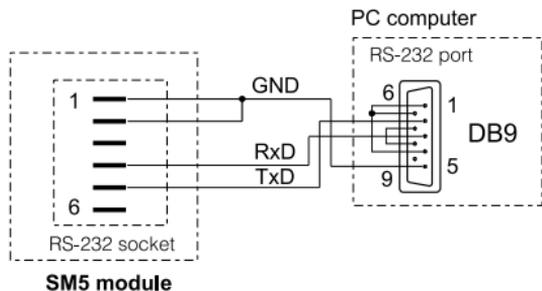
**Fig. 4 Way of the RS-232 interface connection.**
