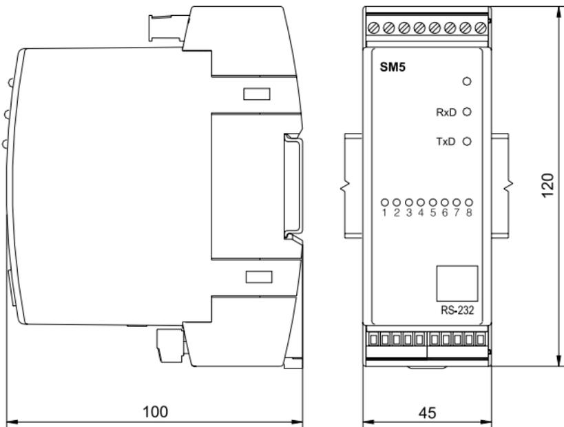
*Fig.1. Overall dimensions and way of the module fixing*
